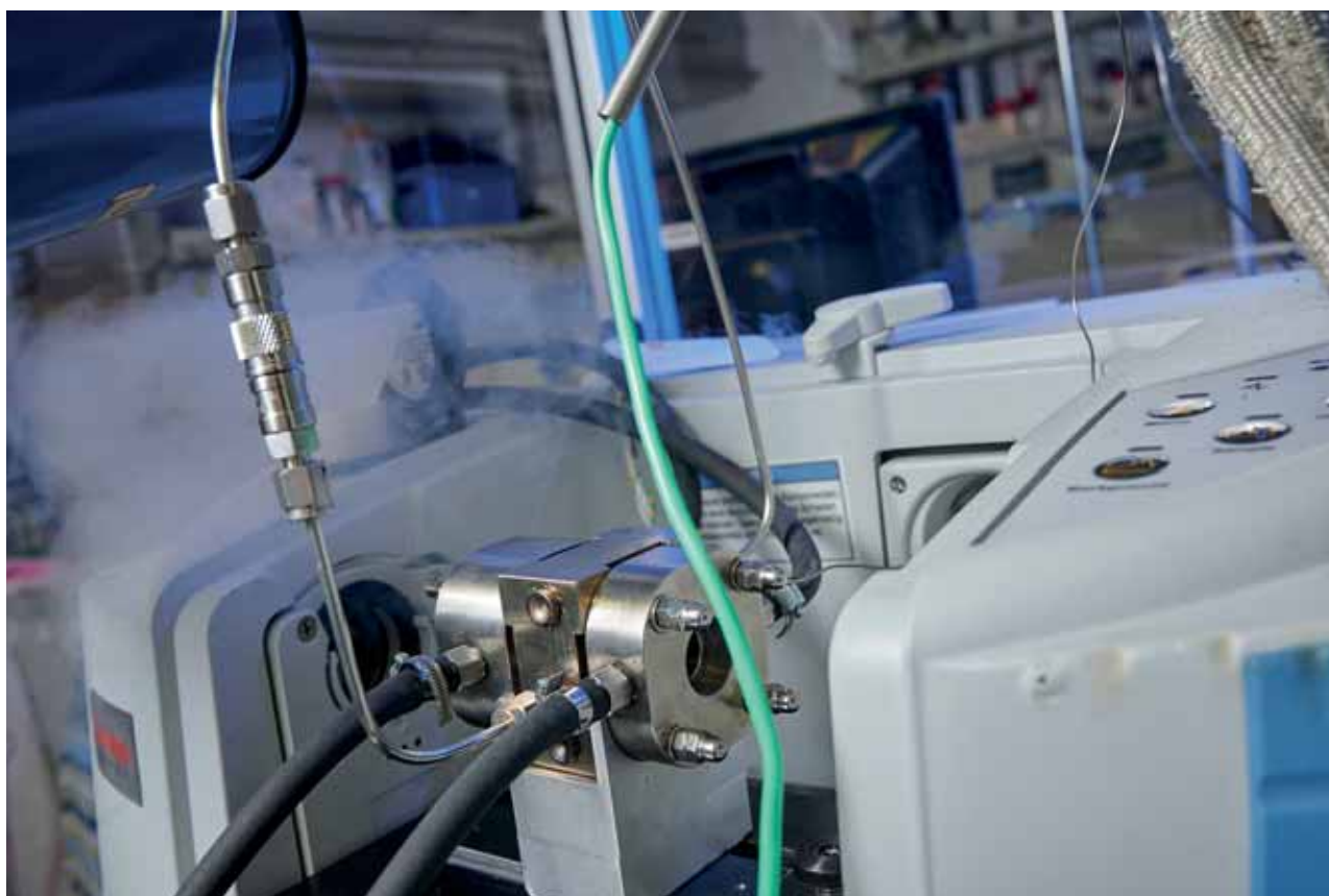
In-house developed cell for operando IR-studies of catalytic material.
