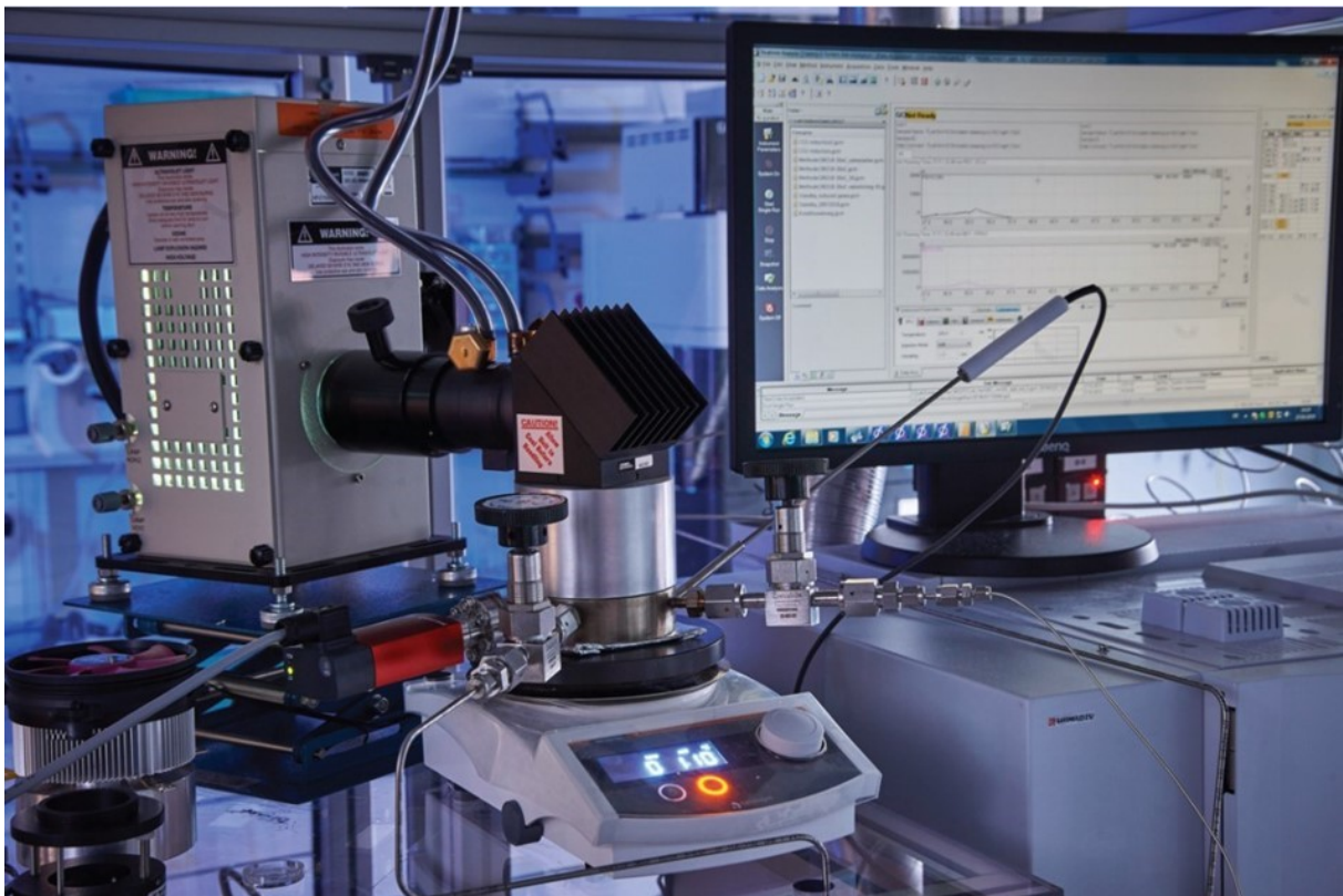
Fig. 1: Photoreactor in the laboratory - Under high-purity conditions, an applied light source (box on the left) activates the photocatalyst in the reactor, allowing the CO 2 to undergo reactions.
