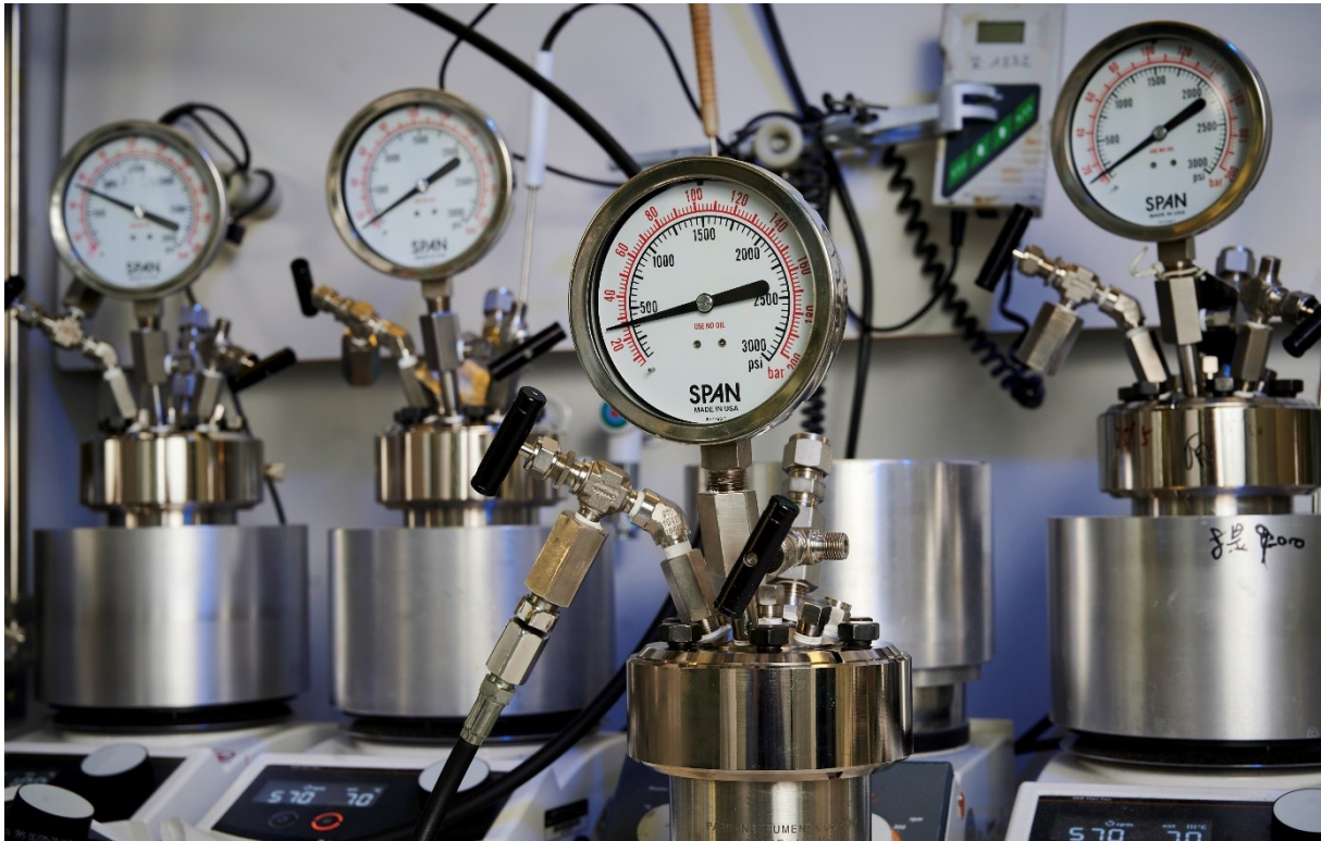
Fig. 1: Methyl formate as hydrogen storage: In these pressurized reactors, the research group studied the release of hydrogen from a methyl formate-water mixture with the aid of a ruthenium catalyst. The amount of hydrogen gas produced in the reactor can be read from the increase in pressure. Photo: LIKAT/Nordlicht
