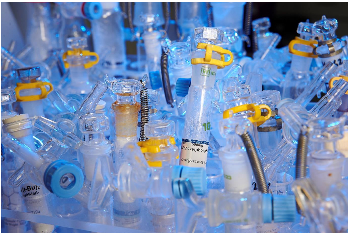
Fig. 1: New air- and water-sensitive catalysts are produced and stored in so-called Schlenk vessels under an inert gas atmosphere. (Picture: LIKAT/Nordlicht)
