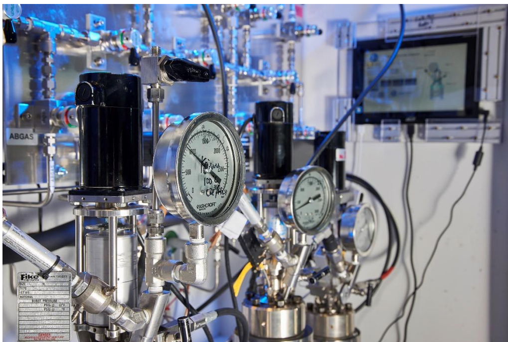
Abb. 1: Pressure reactors at the Leibniz Institute for Catalysis - The reaction is initially carried out on a laboratory scale and is subsequently transferred to a larger scale. (Photo: LIKAT/Nordlicht)
