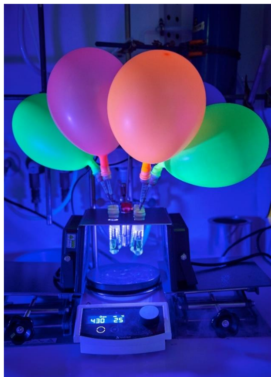
Fig. 2: In the beginning, we simply took balloons, blew them up in the lab and put them over the apparatus." - Experiment with gas entering the reaction vessel .(Nordlicht/LIKAT)
