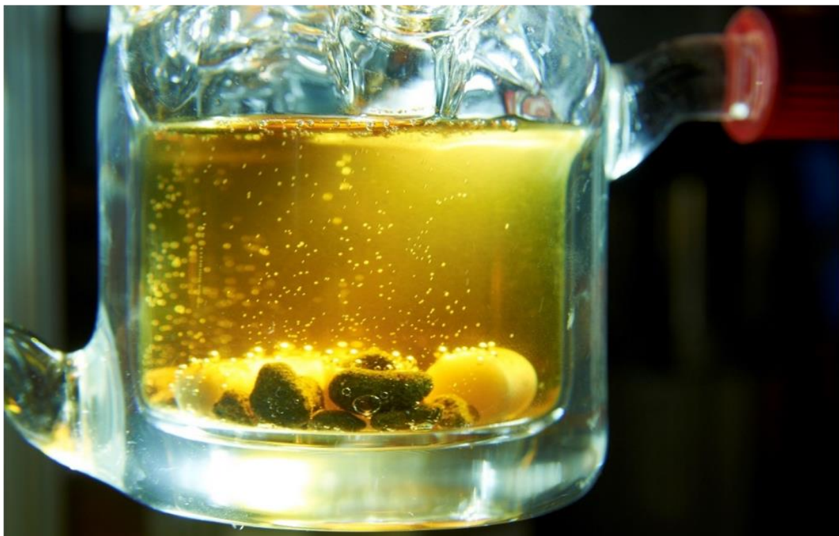
Abb. 2. Top: Cascade reaction - The catalyzed release of hydrogen from an aqueous methanol solution takes place in several steps and passes through various intermediates. Below: Mechanistic investigations are carried out on a laboratory scale; hydrogen release on immobilized catalyst in the reactor.
