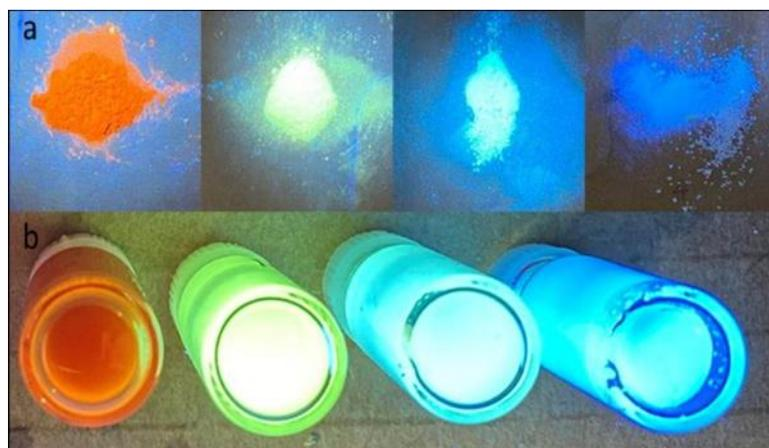
Samples (top row) of the new hybrid photocatalysts spiked with different fluorene scene dyes. Bottom row: samples dispersed in ethanol.
