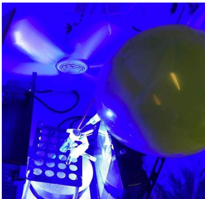
For the laboratory experiment, a reaction for C-H derivatization is irradiated with blue light.
