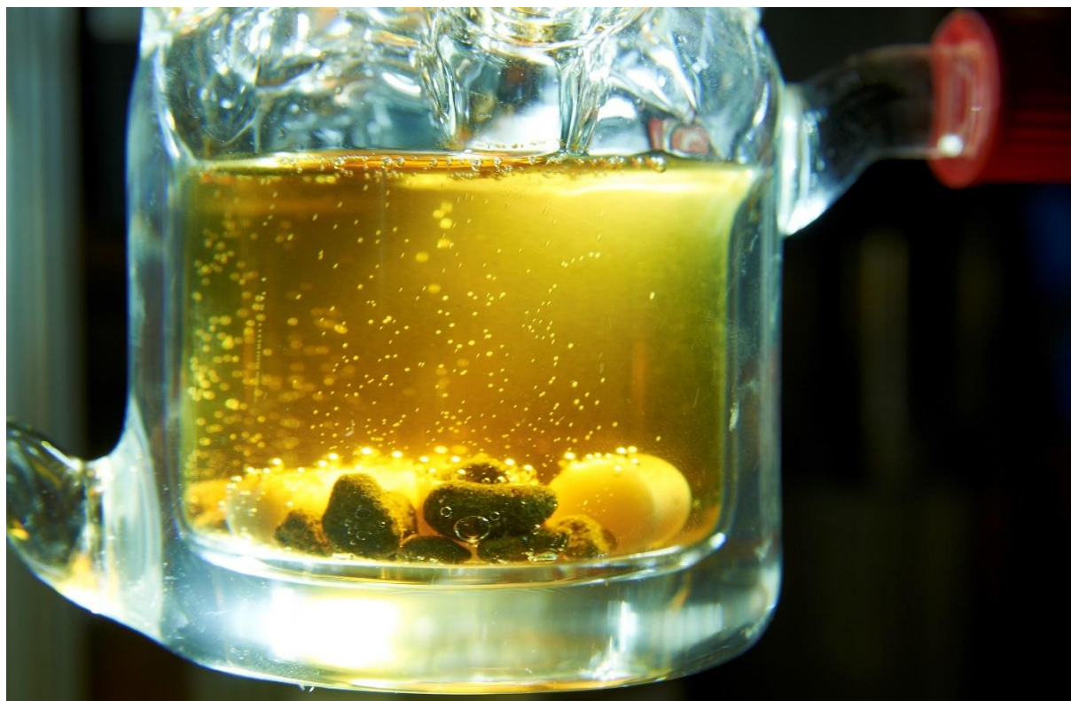
Fig. 2: Mechanistic investigations take place on a laboratory scale; hydrogen release on immobilized catalyst in the reactor ..
